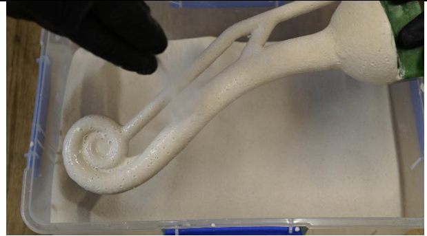
(applying sand to wet coat)
