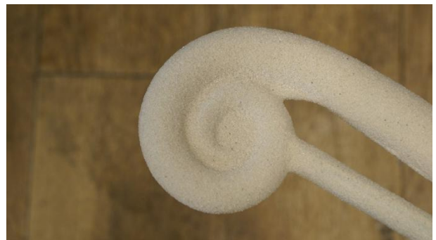
(apply enough sand until the coat has lost its wet glossy appearance)
