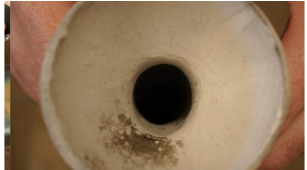
(inspecting shell post-burnout)
