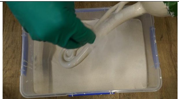
(dusting sand over wet slurry coat)
