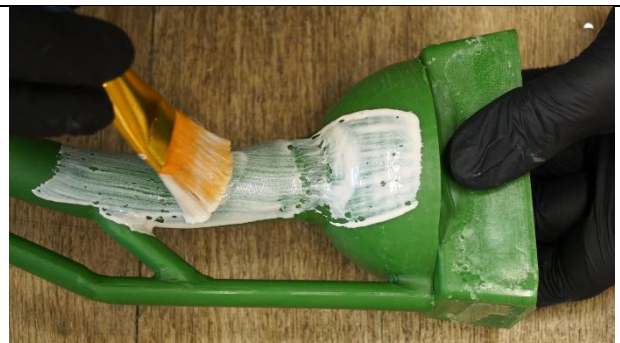
(applying the initial thin coat with a brush)
