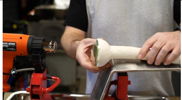
(getting ready to melt wax cup using a hot air gun)
